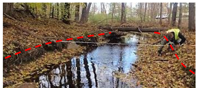
Figure 3-8: Examples of bankfull height indicated by an abrupt transition from bank to floodplain (marked by red lines). (Image adapted with permission from NAACC)
