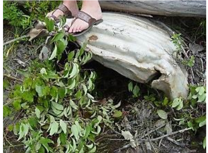
Figure 3-96: An example of a crossing structure with multiple barriers. The culvert is deformed and blocked by debris. (Image credit: NAACC)
